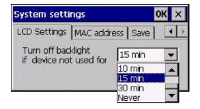
"LCD Settings" page of the **cecp** provides the function to turn off the LCD backlight, and thus elongates the period of service. For example, if the user wants the backlight turned off automatically after 10 minutes when the device was no longer used. The user must select "10 minutes" in the put down box and then press "OK" button. Then the screen save function is enabled. Once the backlight was turned off, events or perturbations from the touch screen can turn it on.
